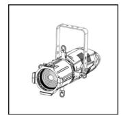
Remove the frontal cap by loosening the upper and lower screws enough to free the cap itself, set the optic's flange tilted about 60°. Insert the optic's flange into the body's receptacle and turn the optic 60° until it is firmly assembled to the projector body, free to rotate but not free to detach itself from the body. Ensure the optic to the body by tightening the two screws previously loosened.
